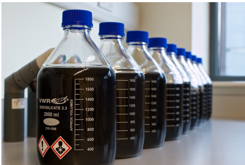
Figure 1: Photo showing large volumes of defect-free graphene dispersions able to be produced.
